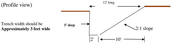
TWO PITS REQUIRED FOR ONE TEST SITE
