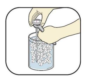
If the display area reads 32°F, the thermometer is accurate.
